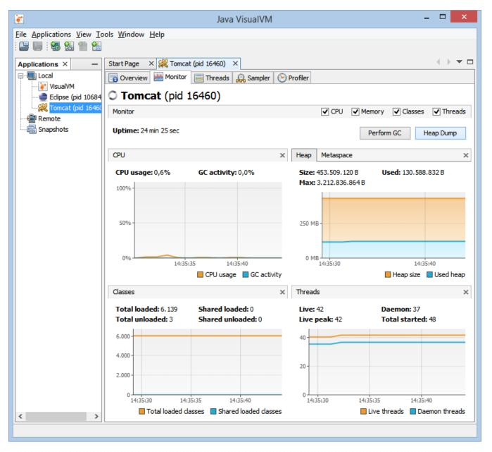
Note that services can't be inspected, so it the process that needs to be inspected is a Servoy Application Server running as a service, the Java process of the Servoy Application Server cannot be inspected. In order to inspect that Servoy Application Server, the service must be stopped and then the Servoy Application Server must be started manually.
